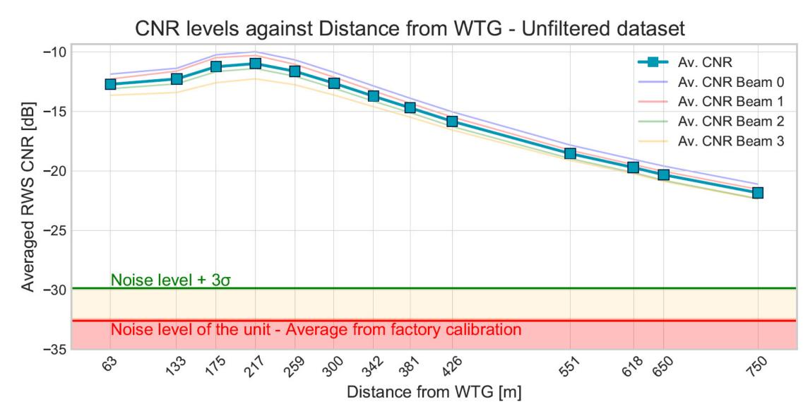
At all ranges, including 750m, the signal is **more than 15dB above the system noise level**. The **CNR peaks near 220m**, which is the chosen focal distance for this long-range lidar.
