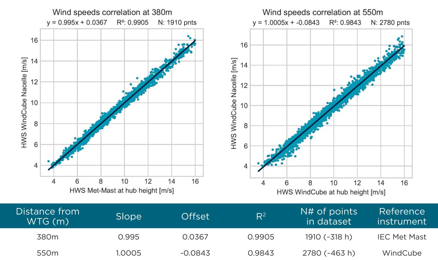
• Correlation between WindCube Nacelle and both references, WindCube and met mast, are as expected. Slope and offset of the linear regressions are in agreement with the nacelle-lidar "white-box" calibration criteria, which is current industry best practice.
